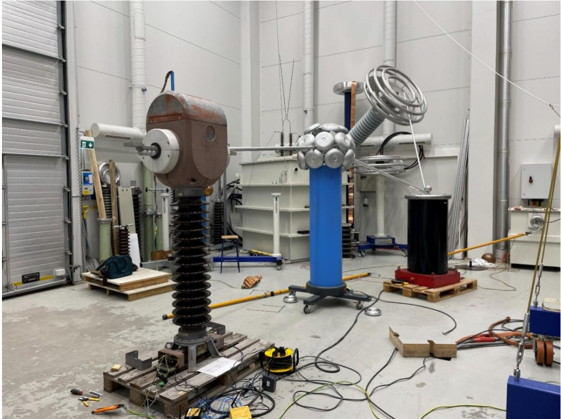
Figure 21. Measurement arrangement for the old CT.
