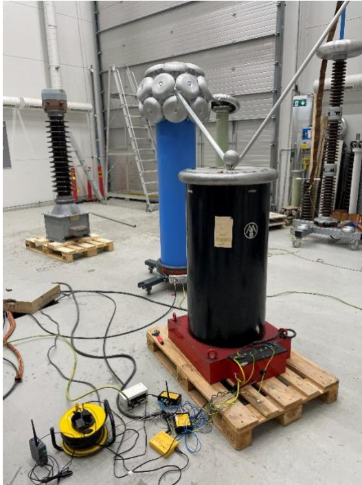
Figure 27. Measurement arrangement for VT from Tampere University.
