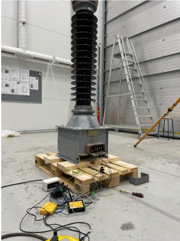
Figure 23. Measurement arrangement for the old VT.
