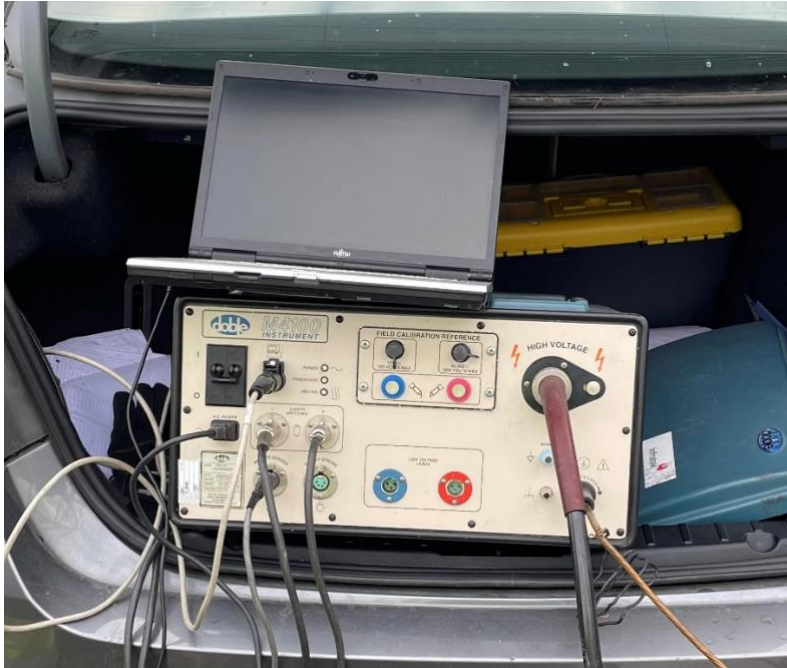
Figure 10. Doble M4100 measurement setup.
