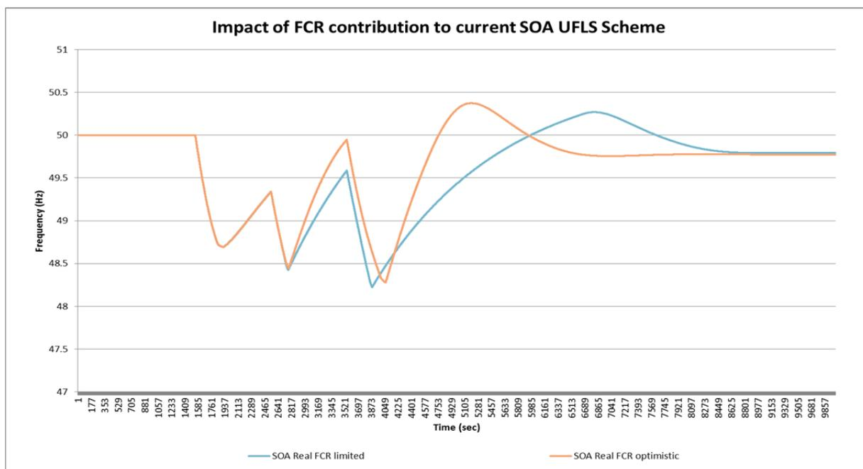
In considering Figure 6 further; as can be seen for the currently implemented UFLS, during the initial stages of generation disconnection, the FCR is capable of sustaining frequency stability thus the FCR levels have limited impact. As the level of available FCR reduces in further disconnection stages the schemes performance is not directly comparable as expected. For this reason it becomes necessary to take a pragmatic view on the levels FCR available in the future.
