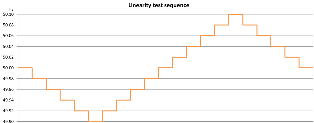
Figure 14. Grid frequency test signal for the FCR-N linearity test for non-continuously controlled reserves.
