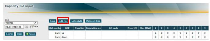
Figure 2 In the Web interface, new bids can be added by clicking on the "add row" button
