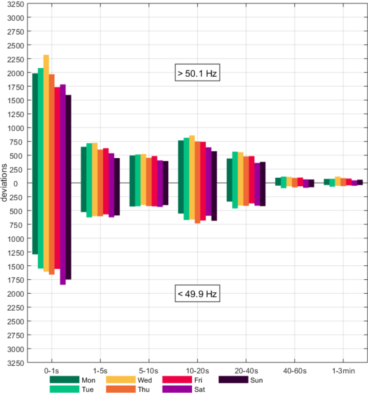
Figure 3.35. Total number of frequency deviations per duration for each day of the week in 2020
