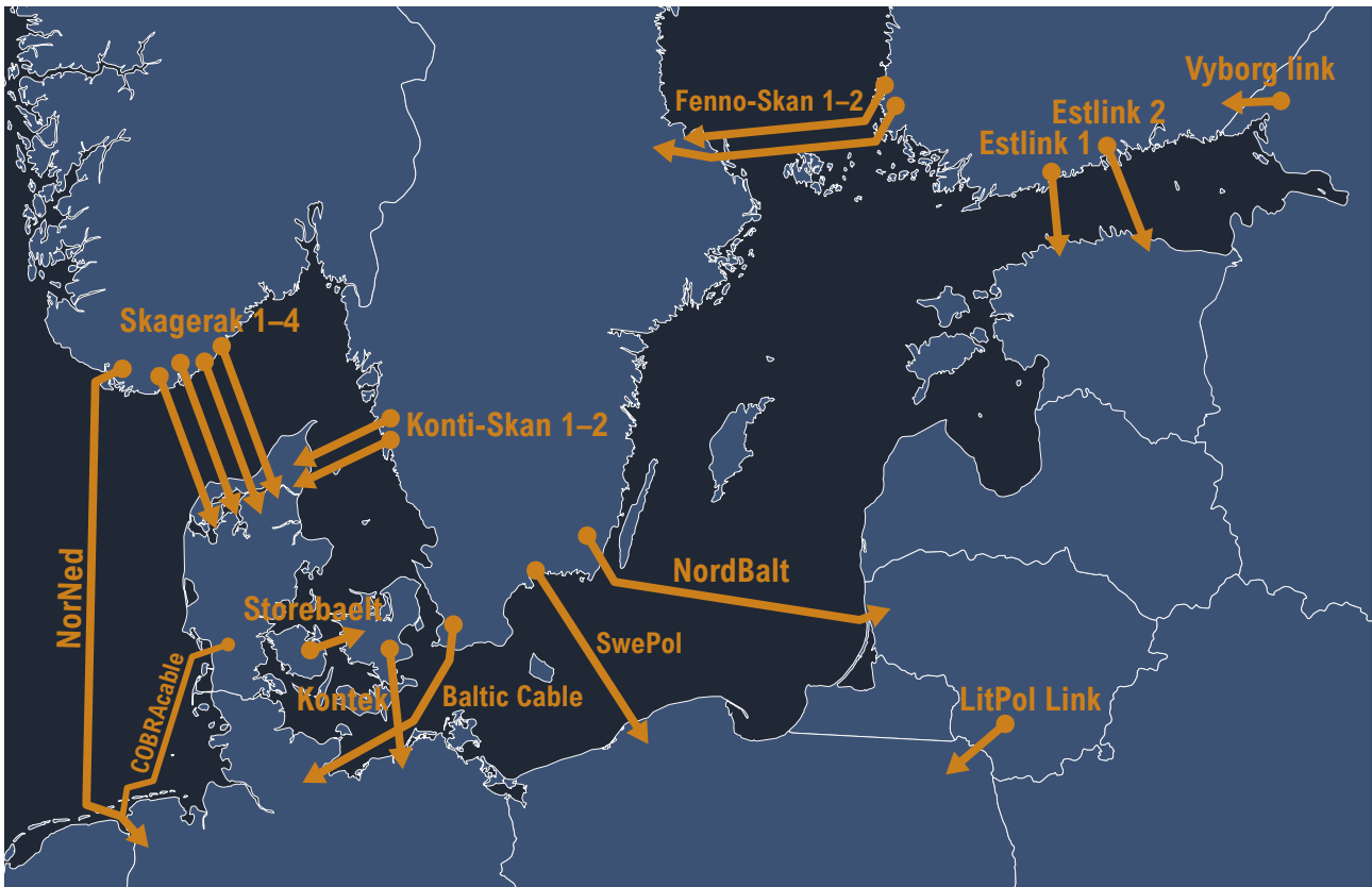
Figure 5.9: A map of the 19 HVDC links included in this report. To distinguish the direction of power flow, each link has a predefined export direction. This direction is indicated by the arrows.
