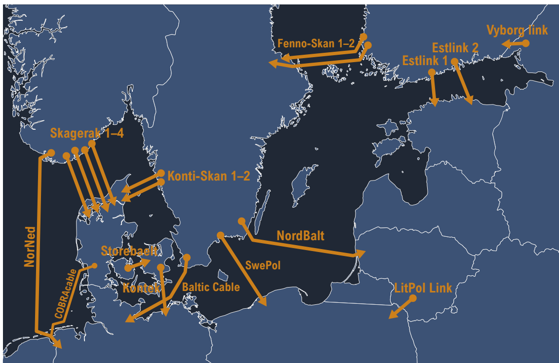
Figure 1.1: A map of the 19 HVDC links included in this report. To distinguish the direction of power flow, each link has a predefined export direction. This direction is indicated by the arrows.
