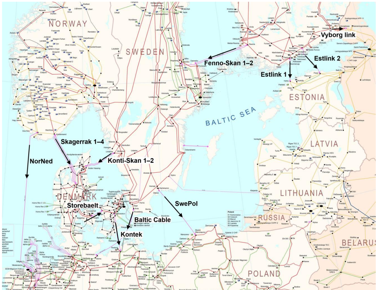
FIGURE 2.1 PART OF THE NORDIC GRID MAP SHOWING THE HVDC LINKS [1]. THE ARROWS INDICATES THE DIRECTION OF EXPORT USED IN THIS REPORT.
