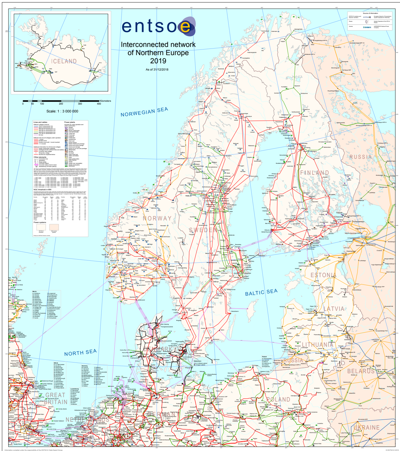
Figure 1.1: The Nordic and Baltic main grids [3] in 2019. The map of 2019 is used because it is the latest available map of interconnected Northern Europe. All of Denmark is included in the disturbance data of this report although only the grid of eastern Denmark belongs to the Nordic synchronous area.
