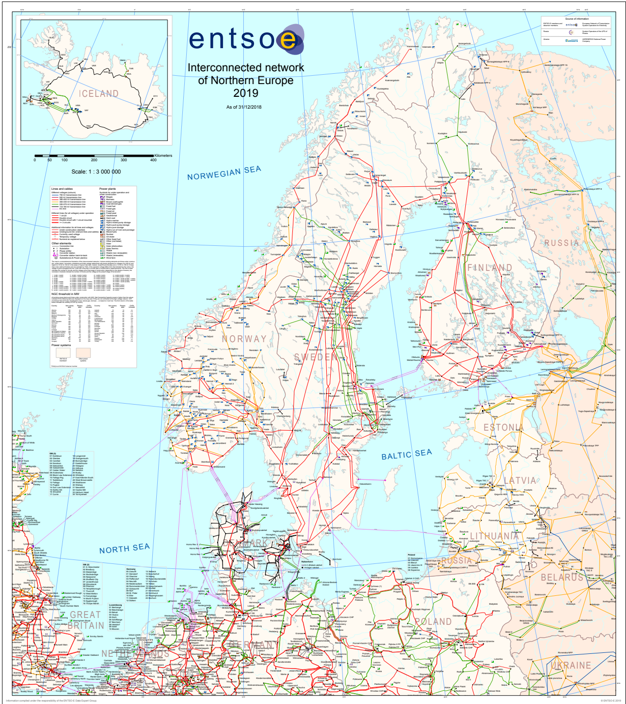
Figure 1.1: The Nordic and Baltic main grids [3]. All of Denmark is included in the disturbance data of this report, although only the grid of eastern Denmark belongs to the Nordic synchronous grid.
